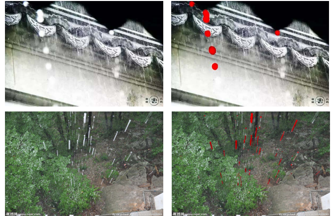
Fig. 2. Examples of rain occlusions in video frames. Compared with additive rain streaks, the rain occlusions (denoted in red color) contain little structural details of the background image.
